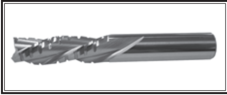
Material Finish-Top: Excellent Material Finish-Bottom: Poor End Point: Endmill Helix Angle: 30°
